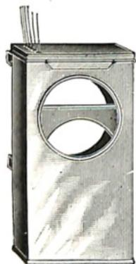
Our Color Box Attachment is made of metal and is equipped with two slide runners, so that it can be slipped on or off very quickly to our spot lamps. Each box contains six color slides, each slide being operated from the outside by pulling a string, which pulls up in place before the light, any color you may desire to show.
