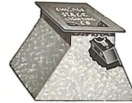
This floor pocket, designed specially for holding our porcelain receptacle No. 691 and plug No. 689, consists of an open bottom sheet iron box equipped with a cast iron floor top with a cable notched hinged drop door.
